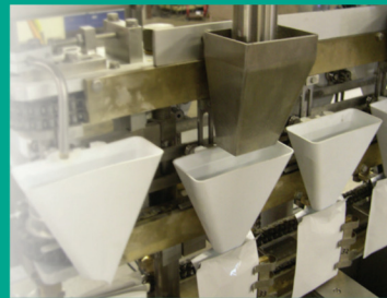
Optional funnel conveyor increases speeds and fill capabilities
