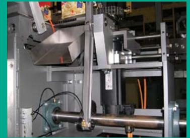
Servo control used for increased precision
